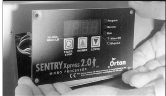
**3** Disconnect the wires from the back of the board. You will find two plugs and two single wires.
