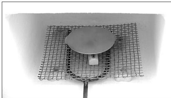
The wire mesh above is referred to as an enameling rack. An enameling fork lifts the rack out of the kiln. A stilt separates the piece from the rack.
