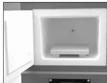
directly on the firing chamber bottom. Use a ceramic shelf on short posts to protect the bottom from glaze drips, glass and enameling powder.
