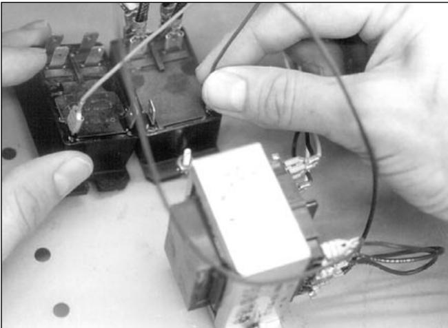
Place the new part next to the old one, aligned in the same direction. Remove and replace one wire at a time. In the photo, the relay is being replaced. The transformer is the part in the foreground.
