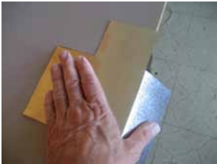
Bend the box over a table edge or similar shape. No tools needed.
