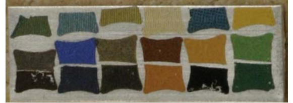
Up: before firing down: after firing at 770C Not all colors remain. Red and purple are gone.
